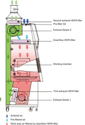
Exhaust air in cabinet duct after filtered by first exhaust HEPA fitter Exhaust air to environment filtered by second exhaust HEPA fitter
