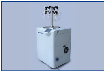
1, 8-manifold bottle hanging device
