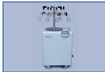
2, 12-manifold bottle hanging device
