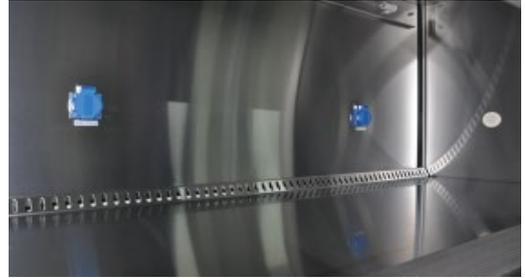
▶ Work table is made by SUS304 plate and can be taken out.
