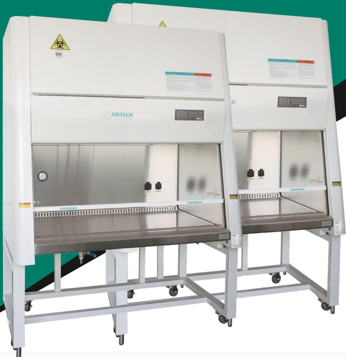
Airtech Biological safety cabinet Class IIA2 airflow ratio is 70% recirculation and 30% exhaust, providing the protection to person, samples and environment from biological hazards and contamination.
