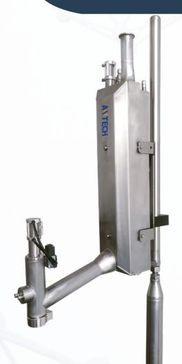
CryoFiller automatic liquid nitrogen filling system is designed to inject LN2 into containers at required pace. After filling into container, liquid nitrogen vaporizes to nitrogen gas and expel air out of container. As a result, oxygen and humidity concentration are reduced, and a suitable pressure is built in container.
