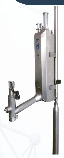
CryoFiller automatic liquid nitrogen filling system is designed to inject LN2 into containers at required pace. After filling into container, liquid nitrogen vaporizes to nitrogen gas and expel air out of container. As a result, oxygen and humidity concentration are reduced, and a suitable pressure is built in container.
