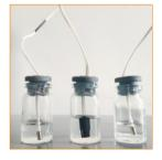
The ultra-fine probes with flexible PTFE wire harness is compact, highly resistant to interference, corrosion-resistant, and easy to calibrate.
