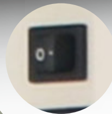
▶ Switch for backup battery
